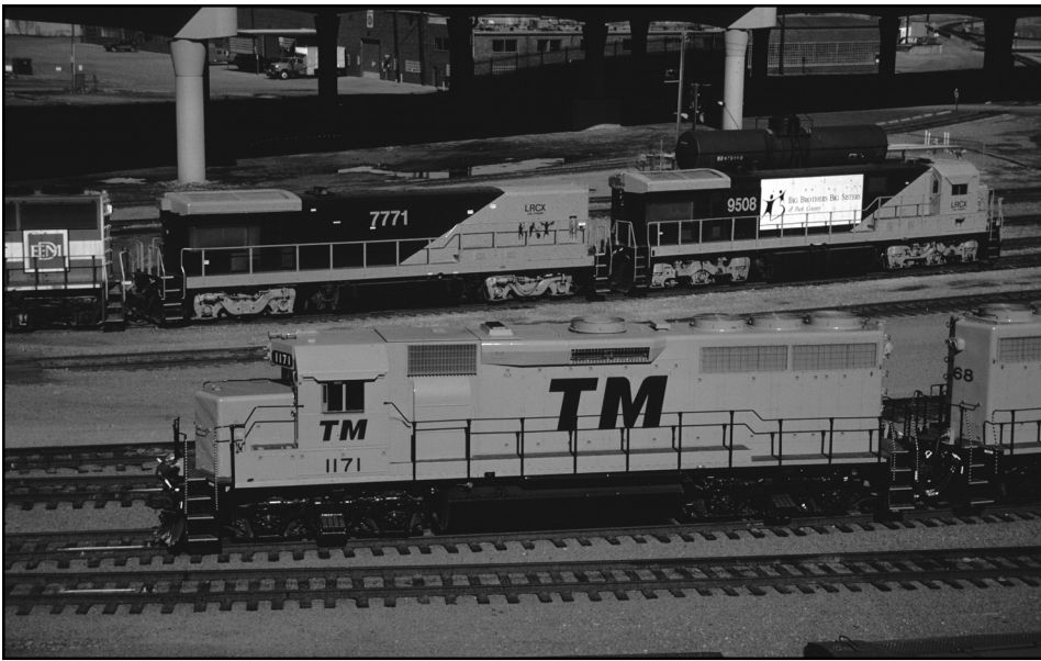
Boise Locomotive GP40-3's #1171 & 1168 are fresh from Idaho at BNSF's Denver Diesel Shop on 4-5-98. Fresh from the Livingston Rebuild Center (LRCX reporting marks) were ex-ATSF SF30C now LRCX 9508 and ex-Cotton Belt B36B-7 now LRCX #7771. The LRCX 9508 sports a sign reading "Big Brothers, Big Sisters of Park County." – Photo by Chip Sherman
